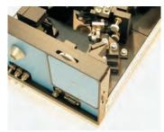
© superfine-precision adjustments of the pump beam, which allow the user to restore quickly the laser generation parameters when the pump beam changes position; for the convenience of use these controls are accessible from the front flange of the laser without opening the case cover
